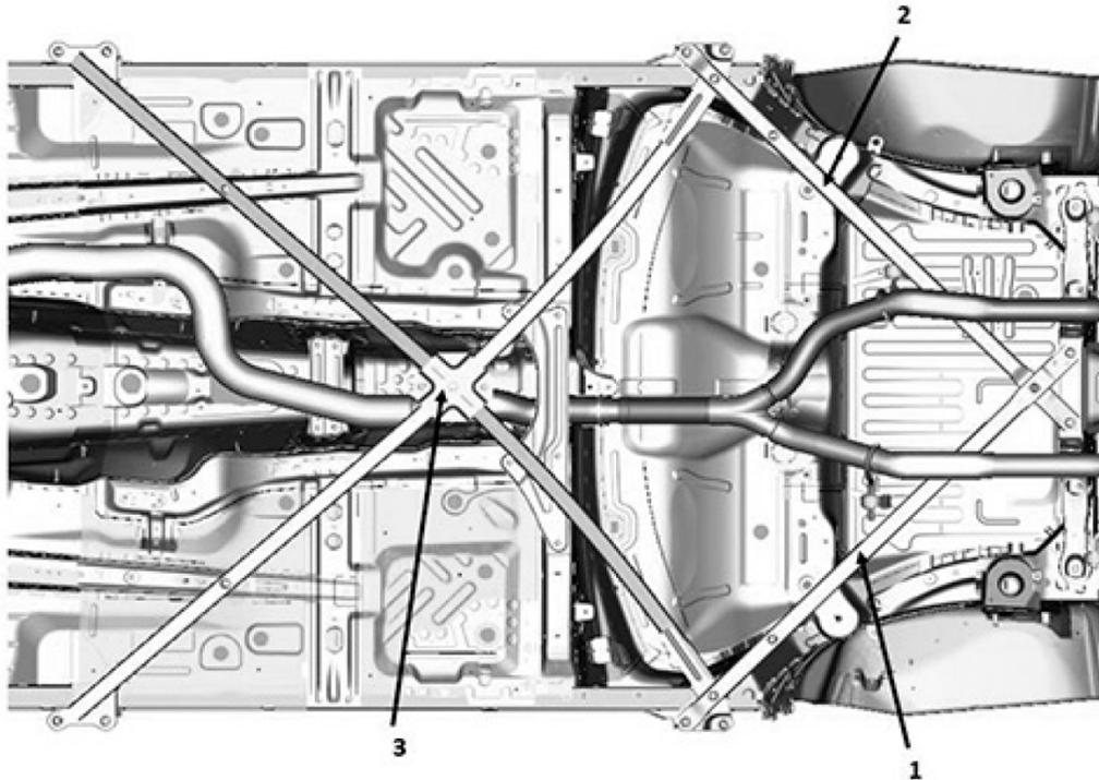
1. **Brace Removal:** For convertible vehicles, it is recommended that you remove the underbody bracing before replacing the accessory exhaust. Remove the braces in the order shown. Retain all fasteners for re-installation.
