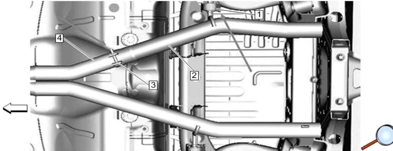
6. **Mid-Pipe Installation:** Install mid-pipe (2) onto Y-pipe (4) with clamp (3). Seat hanger into grommet (1). Do not tighten clamp.
