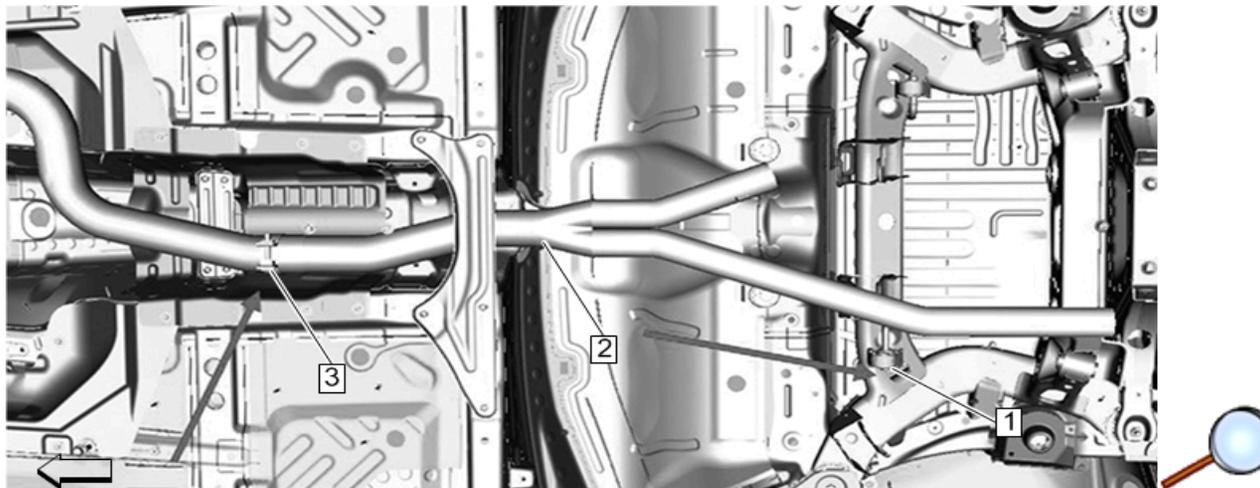
5. **Y-Pipe Installation:** Install Y-pipe (2) onto stock section. Loosely install clamp (3) and seat hanger into rubber grommet (1). Do not tighten clamp.
