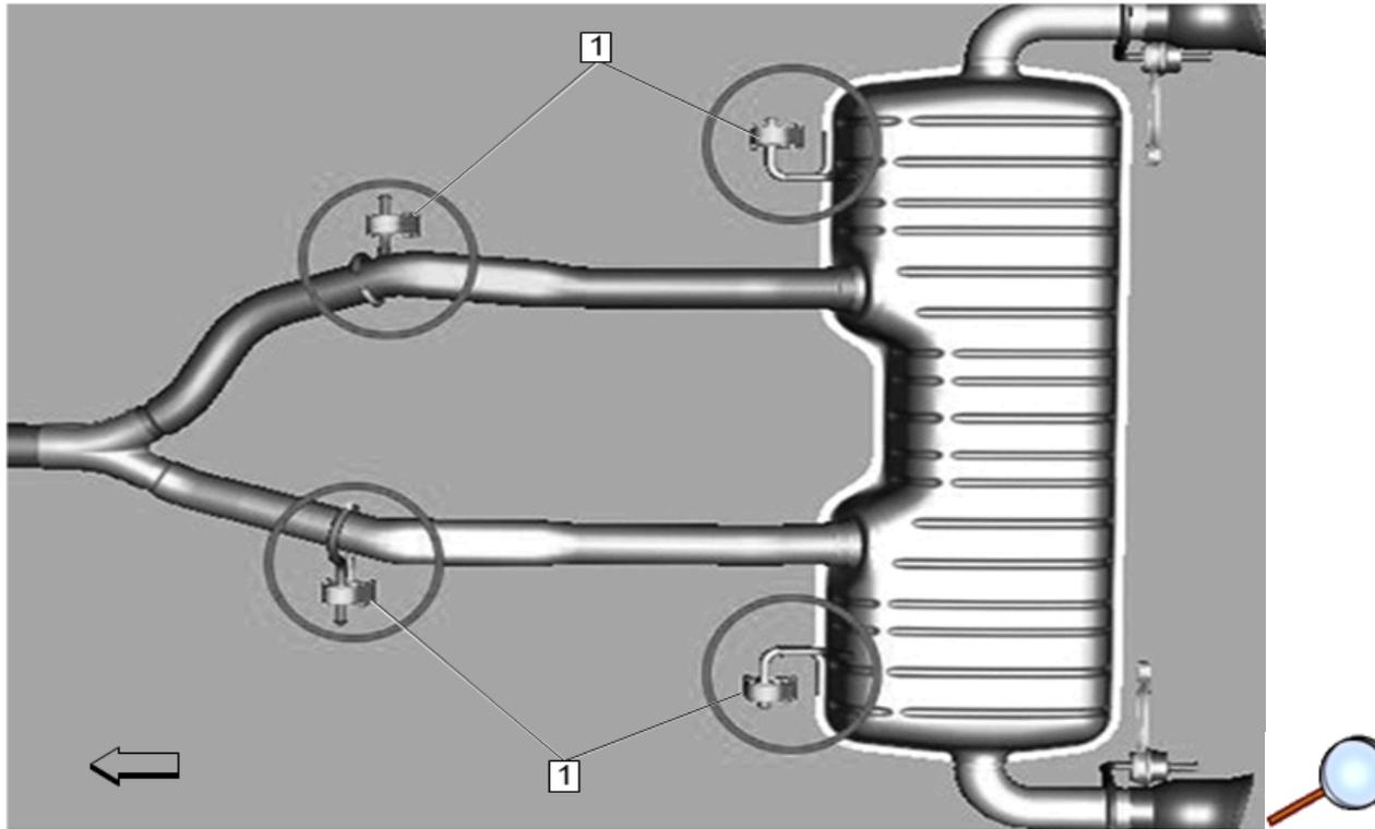
4. **Hanger Locations:** Remove four hangers (1) from mid-section of the rear exhaust and remove rear section.
