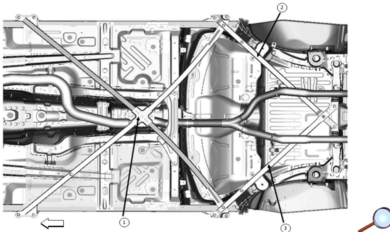
14. **Brace re-attachment order:** Reinstall braces in the order shown. All brace nuts and bolts are torqued 58 Nm (43 lb ft).
