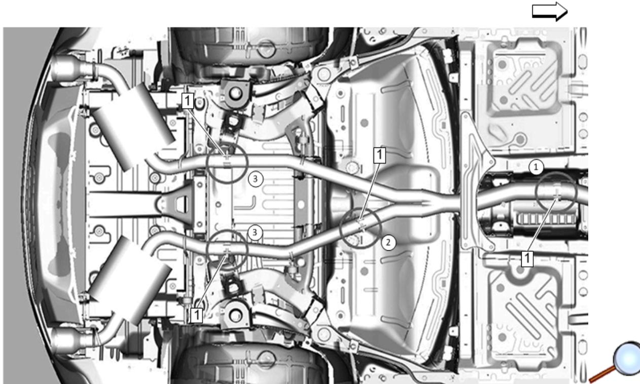
12. **Clamp locations:** Starting at the front and working rearward, tighten the clamps (1) to 45 Nm (33 lb ft).
